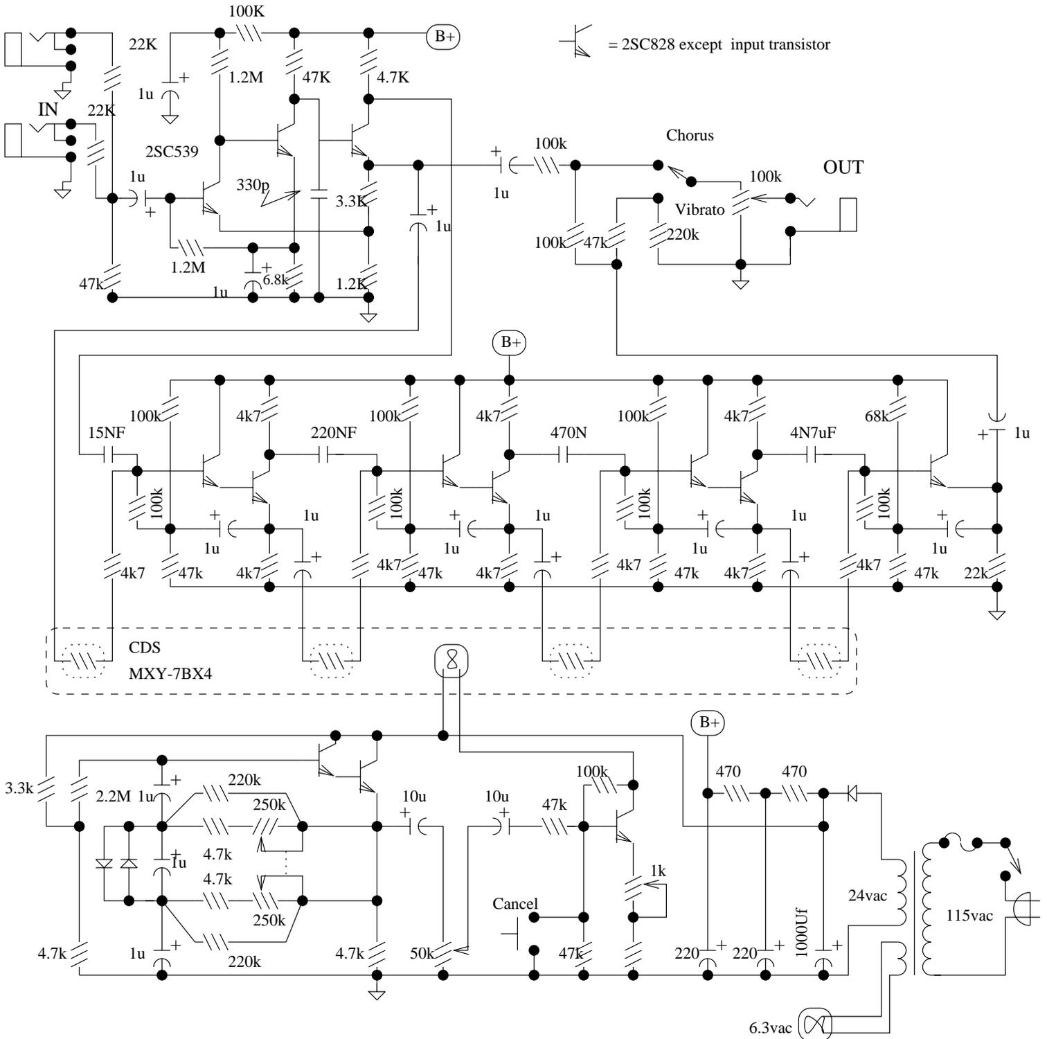
The UniVibe is famous from Jimi's use of it. The LFO is a phase shift oscillator, with the dual 250K pots in the pedal assembly to control speed. A modern version would substitute an LED/photocell optocoupler for the four LDR's and the incandescent light bulb that makes the shifting work. This IS just a four stage phaser, perhaps with some distortion from the signal path thrown in.
